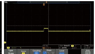
D/D Converter Surge Testing
